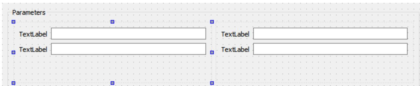
Run the application: distances between labels and line edit boxes does not change but the width of line edit boxes is adjusted. If you do not like it, set the maximum and / or minimum width to proper value.
